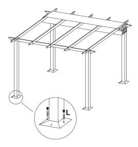
**STEP 14:** Attach legs (E) to floor using bolts (L)
