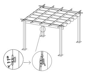
**STEP 11:** Thread cord (O) through runners on beams (C & C1). Follow image below.
