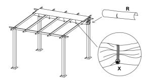
**STEP 15:** Canopy holder (R) can be attached when required to hold canopy in place
