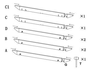
**STEP 1:** Lay out beams (C1, C, D, B & A) and attach decorative end (G) to each end of beams using mallet (T) to gently tap them in
