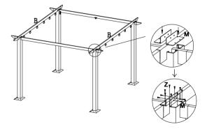
**STEP 5:** Hold leg sections up and attach beams (B) to either end of pergola using mallet (T) to gently tap them in
