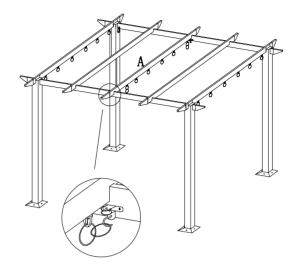
**STEP 8:** Hook double rings (I) to hook on beam (A & C)
