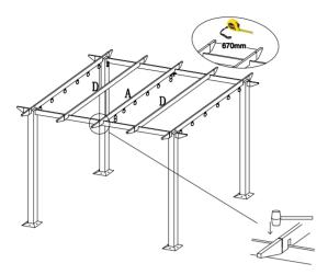
**STEP 7:** Attach beam (A) to centre of pergola and beam (D) on the two sides of (A) using mallet (T) to gently tap them in. Ensure the distance between each beam is about 670MM.
