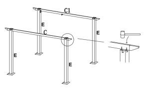
**STEP 3:** Push legs (E) into base plate (H) and using a Philips screwdriver attach the bolts and washer (K)
