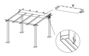
**STEP 13:** Fit canopy cover (U) to top of pergola nearest to beam (C1) so it covers the canopy when closed
