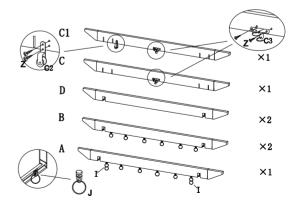
**STEP 2:** Attach the pulleys (C2 & C3) to the beam (C1), and the pulley (C3) to the beam (C) with bolts (Z). Hook single rings (J) to hook on beam (B). Hook double rings(I) on either end of beam(A) and single rings (J) in the middle.
