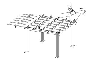
**STEP 10:** Insert canopy supports (F) through and into canopy (Q) attach canopy end supports to canopy supports (N)
