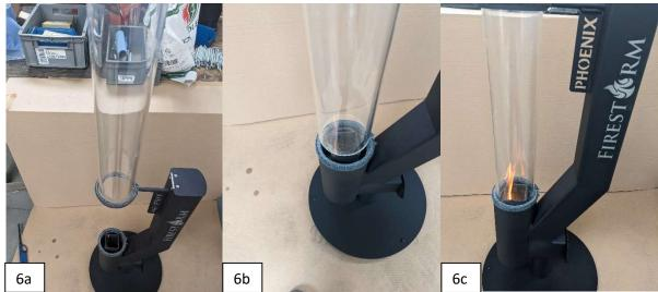
7. Extend the burn time by adding more pellets to the Phoenix through the lid. Important: Make sure the Phoenix does not have less than a quarter of a tube of pellets left before refilling. Refilling beyond this point can choke the fire and cause it to smoke rather than flame. If pellets are not visible in the bottom of the hopper then there is a risk the Phoenix will go out upon refilling.
