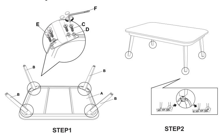
PLEASE ENSURE ALL FIXINGS ARE LEFT LOOSE DURING ASSEMBLY BUT ARE SECURELY TIGHTENED UPON COMPLETION.
