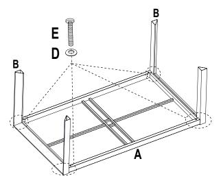
**STEP 1:** Attach Leg (B) to the Table top (A), using the M6x15 Bolt (E) and Washer (D)
