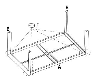
**STEP 2:** Tighten all the bolts on the table,and cover with the Plastic bolt cap (F).
