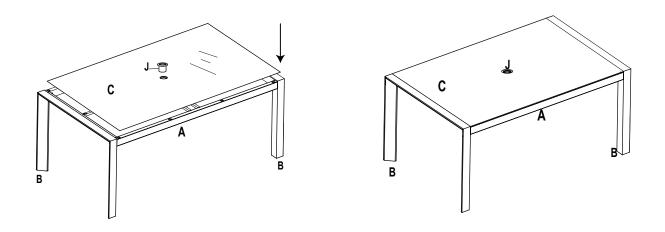
**STEP 3:** Turn the Table over and place the Glass (C) onto the Table, then place the Parasol Bung, Reducer Ring & Cap(J) into the hole
