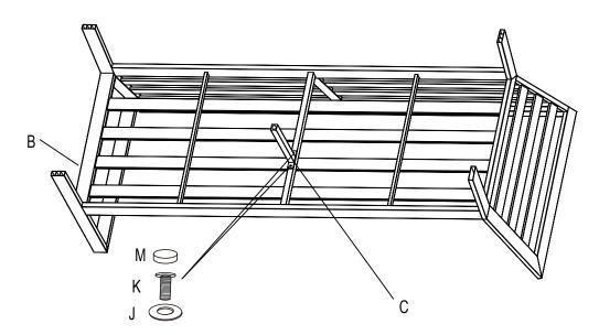
**STEP 2:** Attach Center leg (C) to the Frame 2 (B) using the M6x20 Bolt (K) and Washer (J), tighten and cover with the Plastic bolt cap (M). Turn the sofa over.
