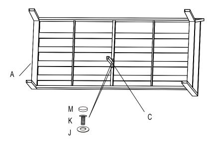
**STEP 1:** Attach Center leg (C) to the Frame 1 (A) using the M6x20 Bolt (K) and Washer (J), tighten and cover with the Plastic bolt cap (M). Turn the sofa over.
