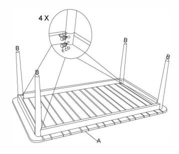
STEP1: Attach Leg (B) to the Table top (A), using the Bolt M6X20 (C) and Washer (D)
