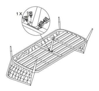
**STEP1:** Attach Center leg (I) to the Frame (H), using the Bolt M6X20 (C) and Washer (D). Tighten the bolts and cover with the Plastic bolt cap (E)
